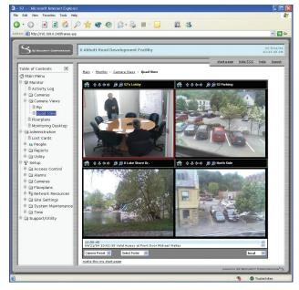
access control, alarm monitoring, temperature monitoring, video and intercom. The appliance allows facilities of all sizes to manage their physical security from any place across an IP network using nothing more than an Internet browser.
