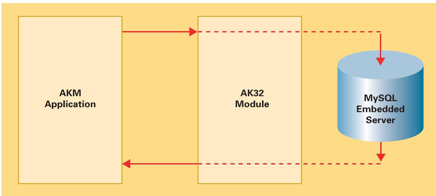
Danfoss' AKM application continuously interacts with a module AK32. This is the interface between AKM and the database. Whenever Danfoss performs a certain operation in AKM that involves data interactions, the application sends out a generalized query to AK32. AK32, in turn, forms the actual query regarding all relevant data and sends it to the MySQL embedded database. AK32 retrieves the requested data in order to return it to the AKM application.
